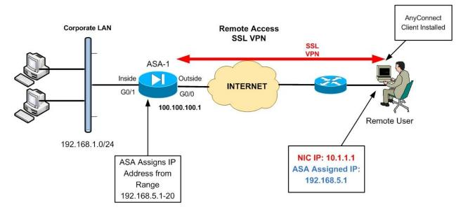
From the diagram above, the ASA firewall is configured as AnyConnect WebVPN server. A remote user has access to the Internet and has an IP address on his/her laptop interface card of 10.1.1.1 (NIC IP). The user can also be behind a router doing NAT/PAT and have his private IP address
