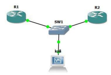
In above topology I will assume you configured R1&R2 with IPsec VPN site-to-site and any necessary static routes
