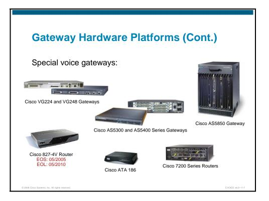
To fit special needs within the customer unified messaging system, Cisco offers standalone voice gateways for specific purposes. Each of these voice gateways fulfills a different need, such as the integration of analog devices into the unified messaging system, enhanced performance, business-class functionality, adaptability, serviceability, and manageability.
