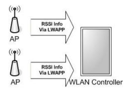
In turn, the WLAN Controller will send the RSSI information it receives from the APs to the Location Appliance. That information is sent in a summarized ("aggregated") form.
