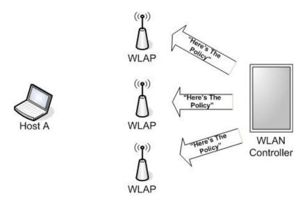
While the lightweight WLAN implementation is generally considered more scalable, note that each implementation type has a centralized point of control.
