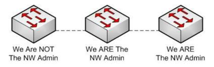
If we're not directly responsible for a switch, we probably don't want to unconditionally trust any values coming in from that switch. That means the trust boundary would not extend to that switch.
