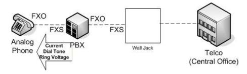
When a Cisco router serves as a gateway, the router will have both FXS and FXO interfaces. The FXO interface will connect a gateway to a Central Office.
