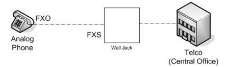
The FXS port will be connected directly to an analog phone or a fax machine, and it supplies vital information to that device, including voltage and dial tone.
