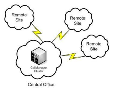
The word "centralized" can also mean "single point of failure", and that's what we have here as far as the remote sites are concerned. The IP Phones at the remote sites will register with the CallManager cluster via the WAN - but what if the WAN link from a remote site goes down? The IP Phones are then cut off from the CallManager cluster.
