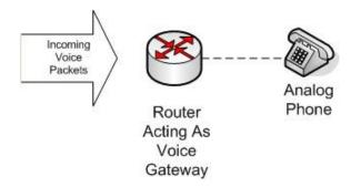
While the router certainly understands what a packet is, the analog phone doesn't know a packet from a hole in the ground. That's a problem. :) It's not enough for the router to forward voice packets to the analog phone; the router has to convert the incoming packets into signals that the analog phone can understand -- namely, an analog signal!
